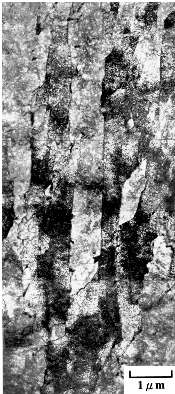
Figure 12 Transmission electron micrographs of a thin foil specimen tempered at 700°C for 20 h.
